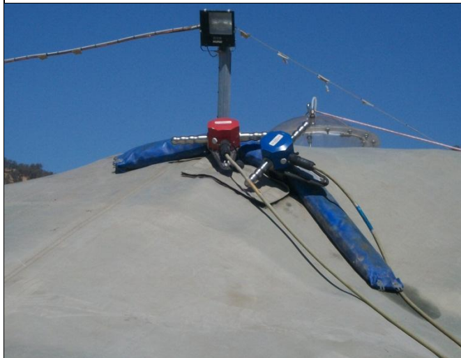
Temperature and oxygen probes inserted into composting material
