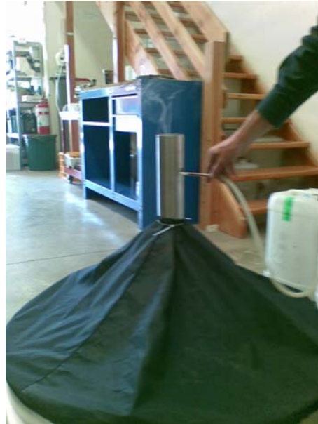
Test 1A (smoke tube showing exit flow)
