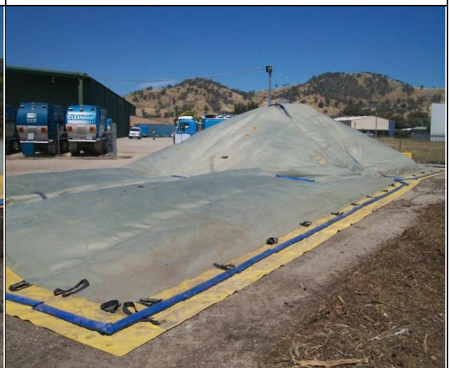
Gore cover with aeration operating (first heap)
